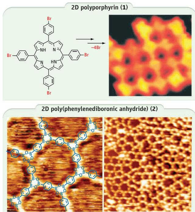
**Conjugated polymers in the plane.** Chemical structures and STM images of (top) polyporphyrin **1** [reproduced from (12), with permission] and (bottom) poly(phenylenediboronic anhydride) **2** [reproduced from (18), with permission] formed on gold surfaces.
